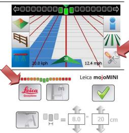
If the **Crosstrack Only Lightbar** is selected, two types of CrossTrack Only lightbar are possible by tapping the button in the bottom left of the screen.
