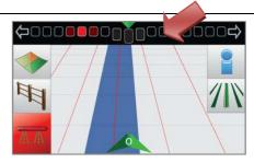
Positioning the vehicle on a previously driven path and tap the **nudge** button.
