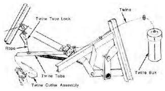
FIGURE 6. Twine Wrapping Mechanism
