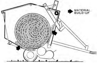
FIGURE 8. Hay Buildup Between Belts.
