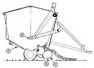
FIGURE 1. Vermeer 605E (A) Bale Forming Belts, (B) Tension Arm, (C) Pickup, (D) Platform Roller.
