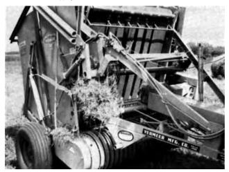
FIGURE 7. Hay Buildup on Twine Wrapping Mechanism.
