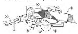
**FIGURE 1.** Vicon MP800 Baler: (1) Power Take-off Shaft, (2) Packer Fingers, (3) Pickup, (4) Auger, (5) Twine Needles, (6) Hydraulic Density Control Cylinders, (7) Knotters, (8) Plunger.
