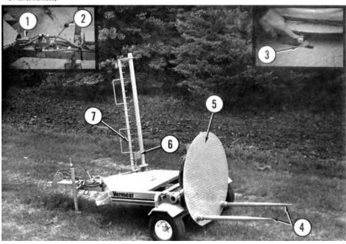
FIGURE 1. Vermeer Bale Wrapper: (1) Bale Position Indicator, (2) Hydraulic Lever, (3) Table Position Trigger, (4) Forks, (5) Table, (6) Brake, (7) Knife.
