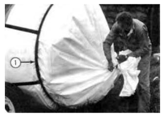
FIGURE 5. Poly Tubing Sleeve End Wrapped and Tied after Installation on Drum; (1) Tension Ring.
