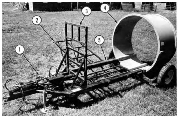
FIGURE 1. Rampak Silage Bagger: (1) Hydraulic Lever, (2) Ramp, (3) Bale Ram, (4) Drum, (5) Carriage
