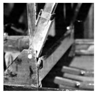
FIGURE 7. Reinforced Drop Extension Rail.
