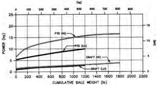
FIGURE 7. Power Consumption During Bale Formation in Alfalfa-Bromegrass (HI)Hard Core - High Density Bale, (LO) Soft Core - Low Density Bale.
