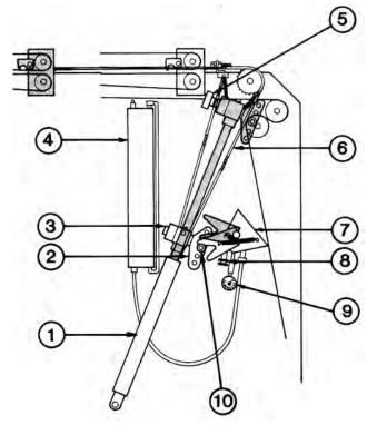
FIGURE 6. Total Density Control System Components: (1) Density Cylinder, (2) Trip Arm, (3) Magnet, (4) Reservoir, (5) Magnetic Sensor, (6) Loading Chain, (7) Valve Trip Mechanism, (8) Adjustable Relief Valve, (9) Pressure Gauge, (10) Trigger.
