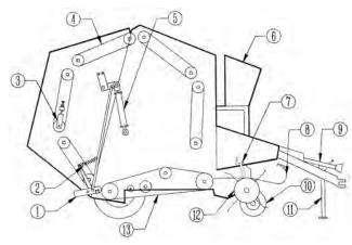
FIGURE 1. New Idea 486 Round Baler: (1) Tailgate Latch, (2) Bale Density Spring, (3) Belt Tension Adjusting Block, (4) Forming Belt, (5) Hydraulic Gate Cylinder, (6) Twine Box, (7) Pickup Transport Arm, (8) Windguard, (9) PTO Drive Shaft, (10) Gauge Wheel, (11) Jack, (12) Pickup, (13) Platform Belt.
