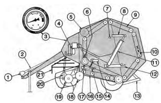
FIGURE 1. Vicon RP 1510/Cl 560 Round Baler: (1) Constant Velocity PTO, (2) Drive Shaft, (3) Density Gauge, (4) Accumulator, (5) Twine Driving Wheel, (6) Automatic Chain Oiler Brushes, (7) Bale Counter, (8) Gate Lock, (9) Upper Forming Belts, (10) Adjusting Block, (11) Gate Cylinder, (12) Gate Latch, (13) Bale Kicker, (14) Chain Idler, (15) Belt Tensioner, (16) Platform Belts, (17) Main Drive Roller, (18) Pickup Pivot Shaft, (19) Pickup, (20) Transport Arm, (21) Pickup Guard.
