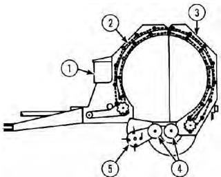
FIGURE 1. Krone KR180 Baler: (1) Twine Box, (2) Bale Forming Chain, (3) Rear Gate, (4) Platform Rollers, (5) Pickup.
