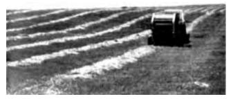
FIGURE 8. Windrow Dropping Out Behind the Baler in Light, Dry Crop Conditions.
