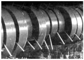
FIGURE 10. Damaged Pickup.
