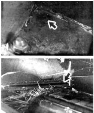
FIGURE 11. Frame Failure: (Upper) Broken Bolt, (Lower) Spreading Between the Front Housing and the Roller Support Bracket.
