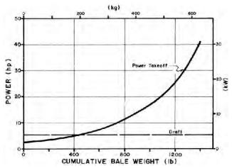
FIGURE 6. Power Consumption During Bale Formation in Alfalfa Bromegrass.
