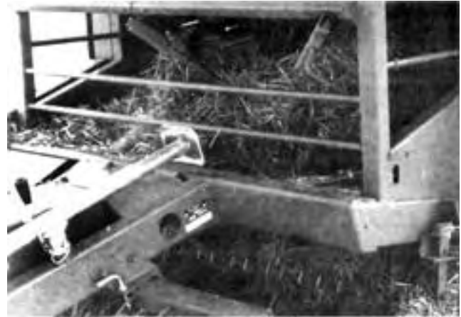
FIGURE 7. Backfeeding of Very Dry, Short Straw into the Pickup Area When the Bale was Nearing Completion.
