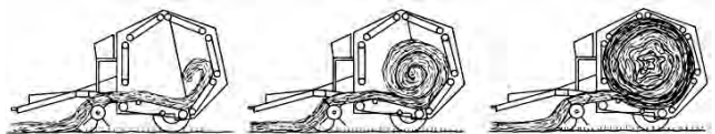
FIGURE 6. Stages of Bale Formation: (Left) Starting Bale, (Centre) Partially Completed Bale, (Right) Completed Bale.
