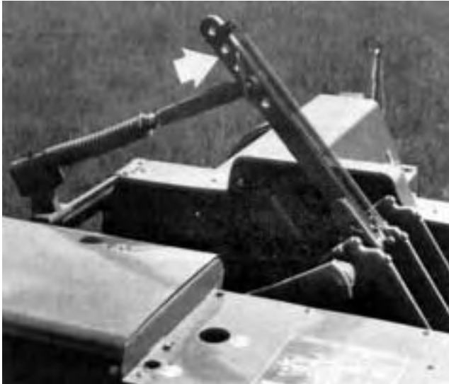
FIGURE 7. Packer Finger Adjustment.
