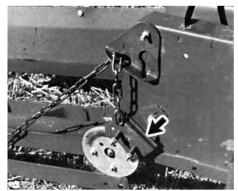
FIGURE 8. Bale Chute Anti-bounce Brake.
