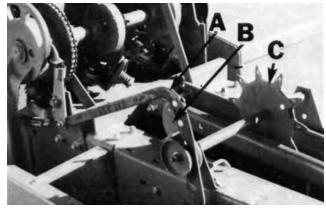
FIGURE 3. Bale Length Adjustment: (A) Metering Arm, (B) Adjustable Stop, (C) Metering Wheel
