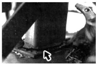
FIGURE 9. Broken Knotter Mounting Frame.
