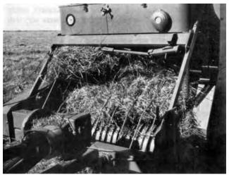
Figure 7. Plugging in Heavy Windrows Due to Excessive Lift of Compression Bars.
