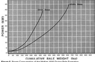
Figure 5. Power Consumption of the McKee 1500 During Bale Formation.
