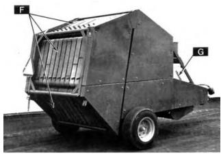
Figure 3. Rear View of McKee 1500 Round Baler. Identification of components: (F) Forming Belts, (G) Pickup Transport Lever. Page 2
