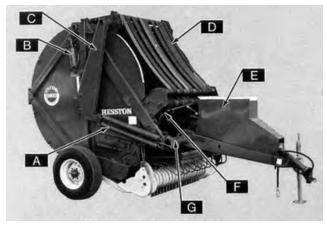
**Figure 2.** Front view of Hesston 5800 Rounder, Identification of Components: (A) Tension Spring, (B) Gate Cylinder, (C) Tension Arm, (D) Forming Belts, (E) Twine Box,(F) Twine Cutter, (G) Pickup Transport Lever.
