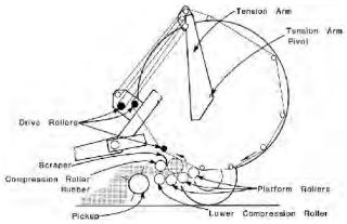
Figure 1. Schematic View of Hesston 5800 Rounder.
