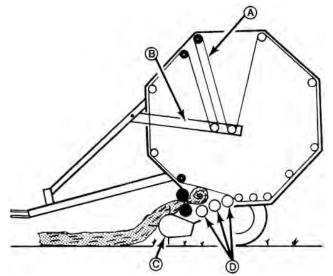
FIGURE 1. Massey-Ferguson MF 560 Baler: (A) Bale Forming Belts, (B) Tension Arm, (C) Pickup, (D) Platform Rollers.
