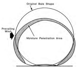
FIGURE 3. A Typical Bale After 100 Days of Weathering.
