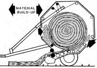
FIGURE 8. Hay Buildup Between Belts.
