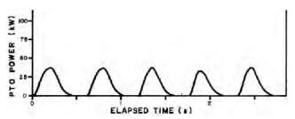
FIGURE 5. Instantaneous Power Take-off Requirements when Baling Alfalfa at 10 t/h Feedrate.
