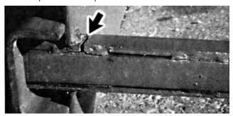
FIGURE 12. Failure of Bale Chute Frame Welds.
