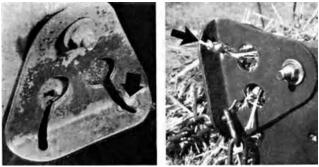
FIGURE 11. Deformed and Cracked Bale Chute Brackets.
