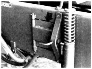
FIGURE 6. Side Resistors.
