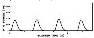
FIGURE 4. Instantaneous Power Take-off Requirements when Baling Alfalfa at 10 t/h Feedrate.
